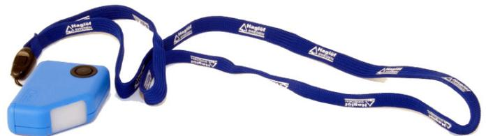
The blue C I is the ideal instrument to measure slopes and inclination of trees, buildings, walls, tunnels, roads and more in a quick way. Field pro's will appreciate the simplicity and accuracy of the C I. Art. no. 15-102-1012, specify deg. or %.
