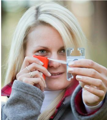
The EC II D-R is an electronic clinometer with a factor gauge and in-built functions to get estimates for basal area and volume. Use the EC II D-R for height readings from any manually measured and input distance or with a calculated distance.
