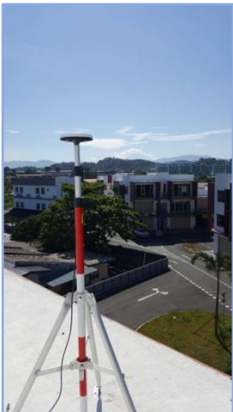
Semi-permanent Reference Station
