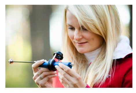
By studying an extracted wood core, you can get access to hidden information on the tree, such as its condition, diseases, growth and age. With high quality optics and rugged construction, the Tree Ring Measurer will be a valuable field instrument that can improve reading of wood cores and the accuracy of your results.
