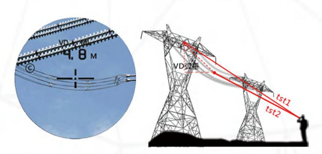
VD ML Separately measure the distance of different wires, and you will know the layer distance Separately measure the distance of connecting place and lowest point of wire you will know the vertical distance.
