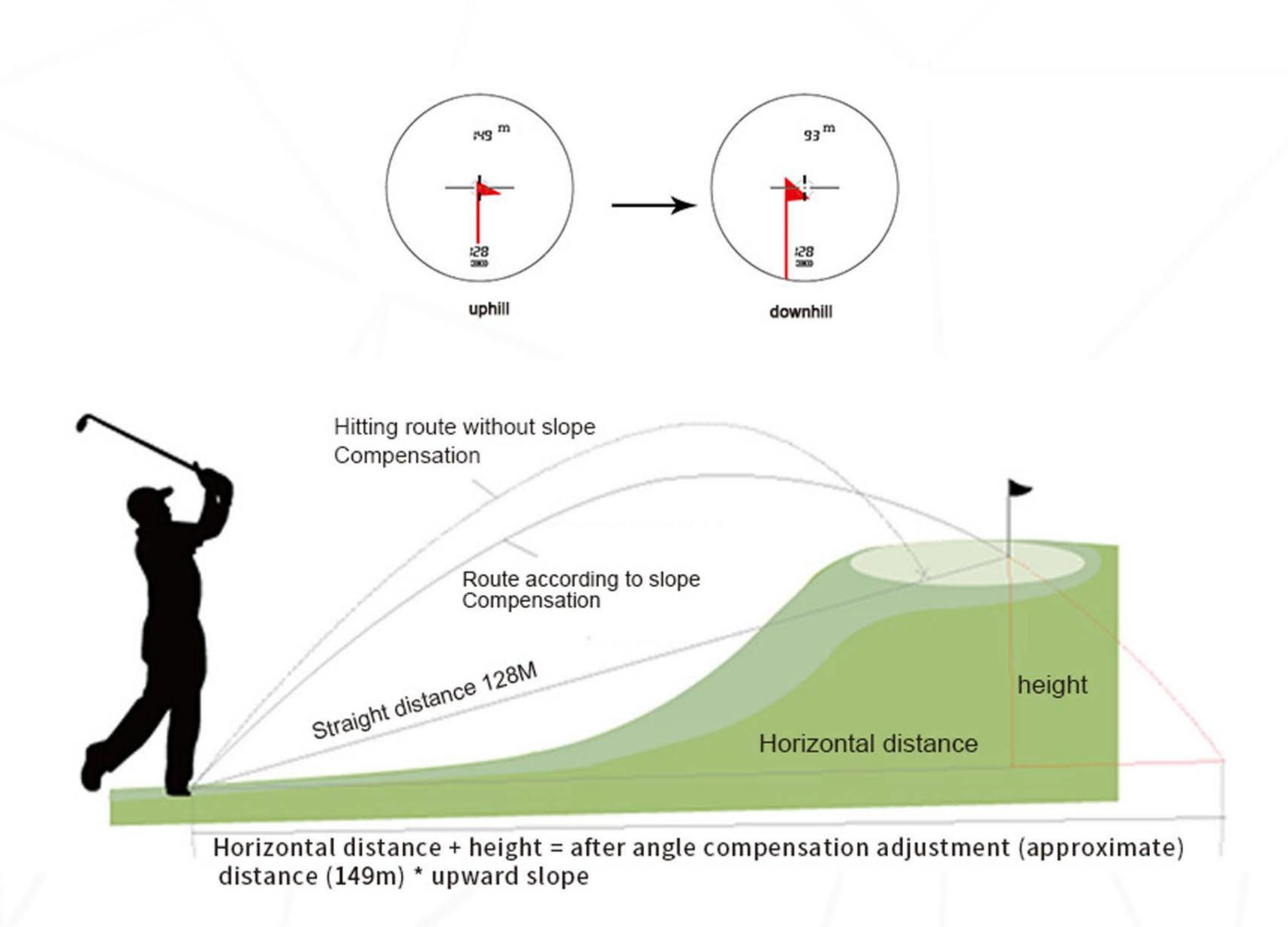
The above figures represent "slope adjustment distance", the following number represents "a straight—line distance", both of which are displayed on the internal display.
