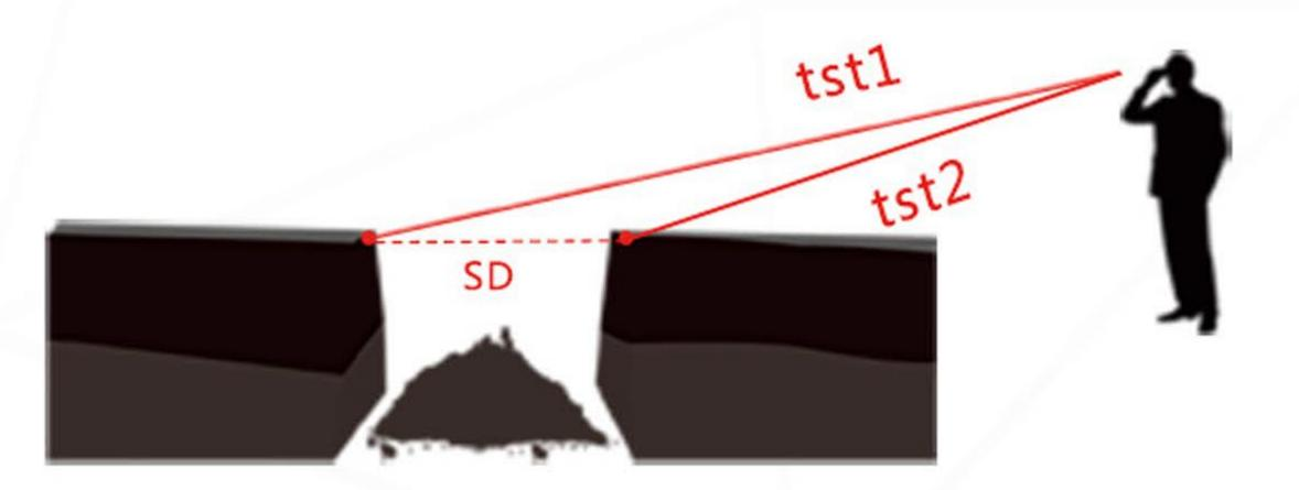
**SD ML** Separately measure the distance from two points of bam breach, you will get the width of breach.
