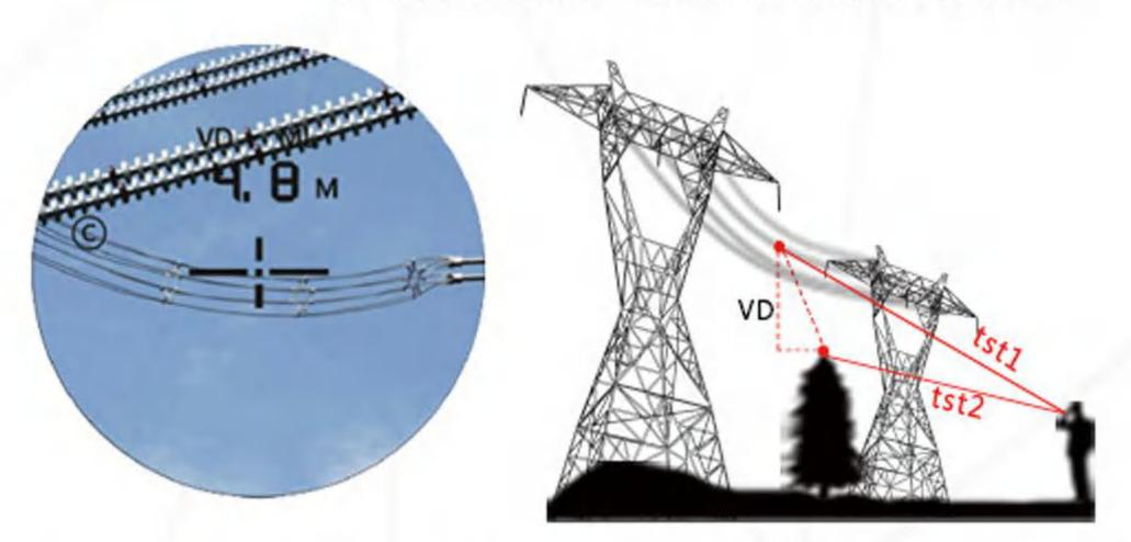
VD ML Separately measure the distance of guy wire of transmission corridor and tree around it, you also can know the vertical height.
