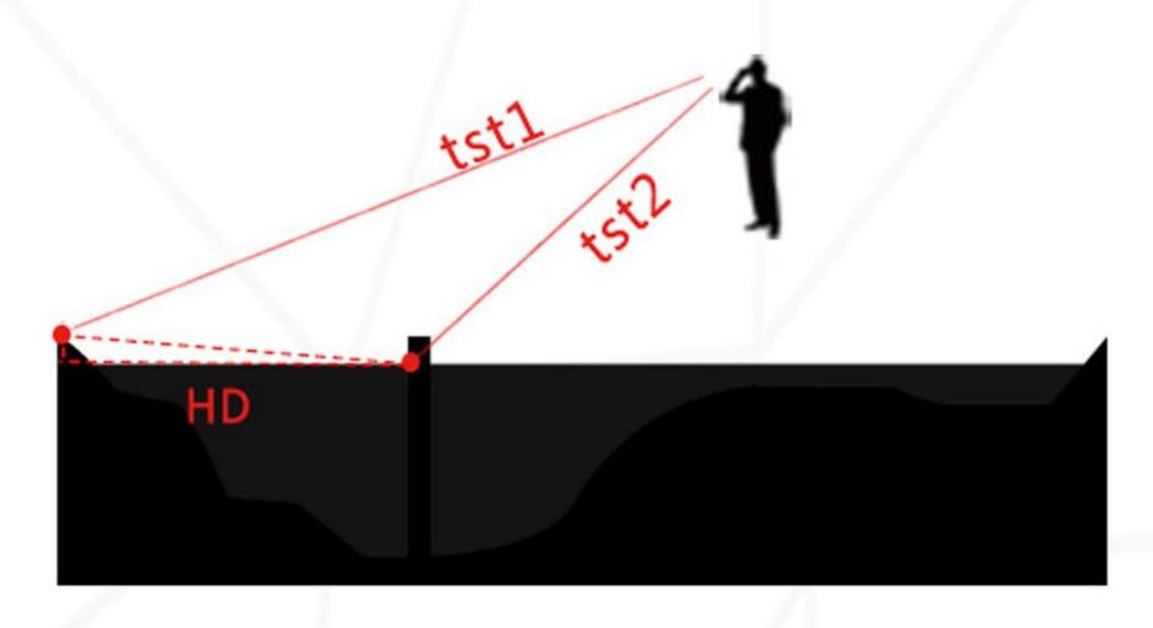
HD ML measure the straight distance of starting pile and the watchpoint
