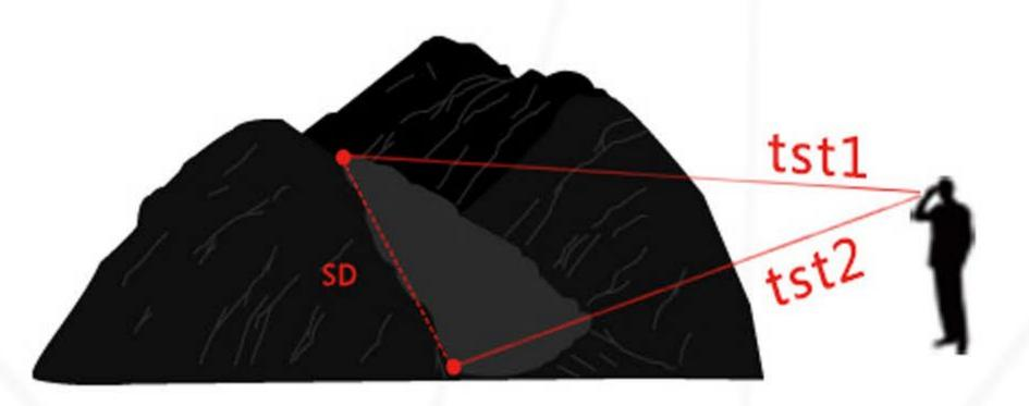
**SD ML** separately measure the two points in mud-rock flow or mount, you will know the length or width.
