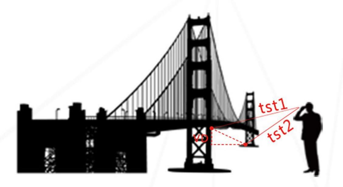
VD ML Separately measure the distance from bottle of bridge and the bottle of piers, you will get the vertical height from water surface.
