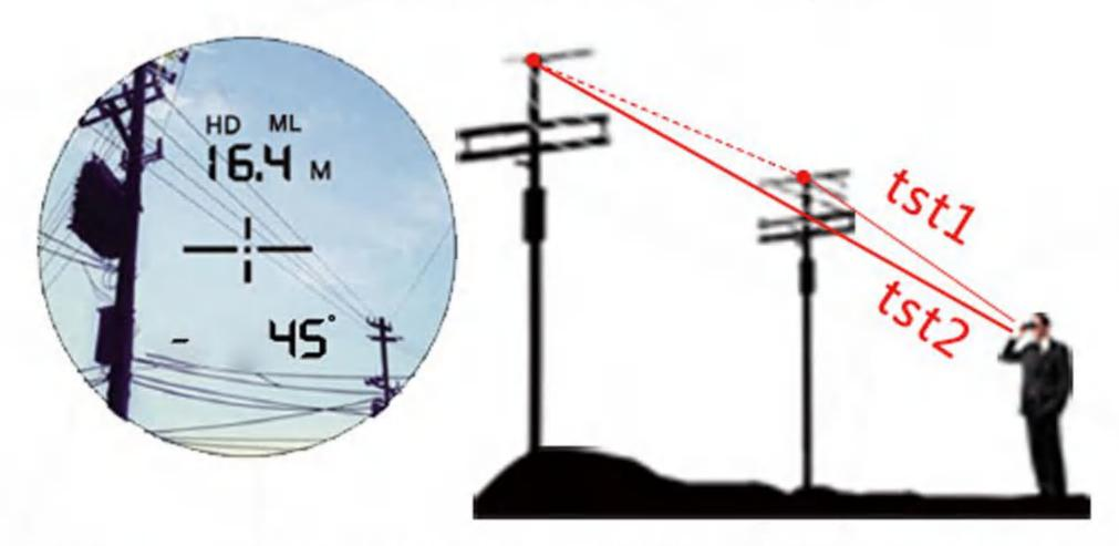
HD ML Separately measure the distance at the same position of two electric power poles such as tst1 and tst2, you will know the distance of this two place (distance of the two electric power pole.
