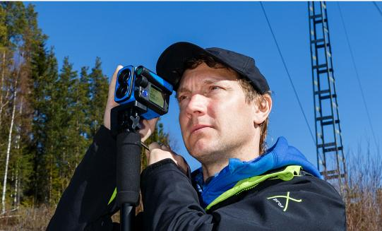
The Laser Geo is a great choice of instrument for control work in utility industry. Hazard trees, border trees and safety distances can be measured and evaluated for accident prevention and to secure power lines, railways and roads. With storing and processing capacities, special functions can be ordered and implemented for targeted user areas.
